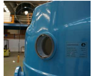
100% full vision inside: Methacrylate sightglasses
