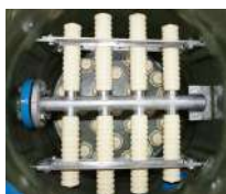
Stainless Steel beams with PP arms
