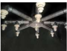
Stainless Steel star with PP nozzles
